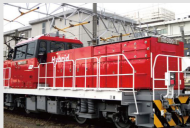
Japan Freight Railway Hybrid shunting engine which commenced operations in 2012.
