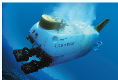
Shinkai 6500 Submarine A crewed research submersible capable of diving to depths of 6,500 metres.
